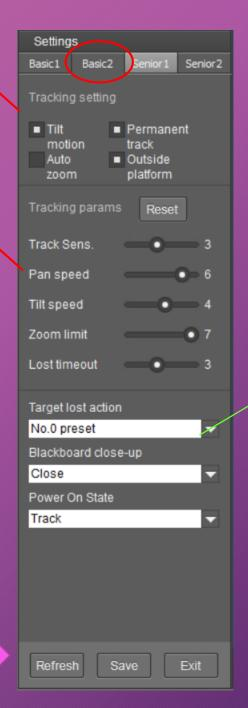
Set Target lost to 0 or 1. This references the previous set presets. NOTE: "Auto tracking settings" references the small lower tracking camera not the PTZ camera reference.
