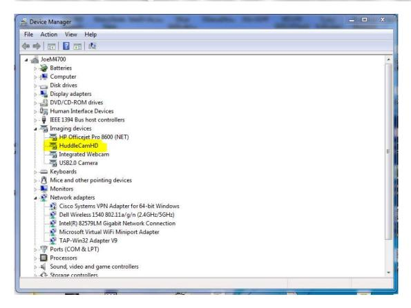
In this example, you can see the HuddleCam model in use connected as a fully functional USB 3.0 device (HuddleCamHD) as well as a USB 2.0 device with limited functionality (USB2.0 Camera).
