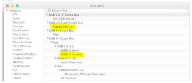
In this example, you can see the HuddleCam model in use connected as a fully functional USB 3.0 device "HuddleCamHD" as well as a "USB2.0 camera" with limited functionality (USB2.0 camera).
